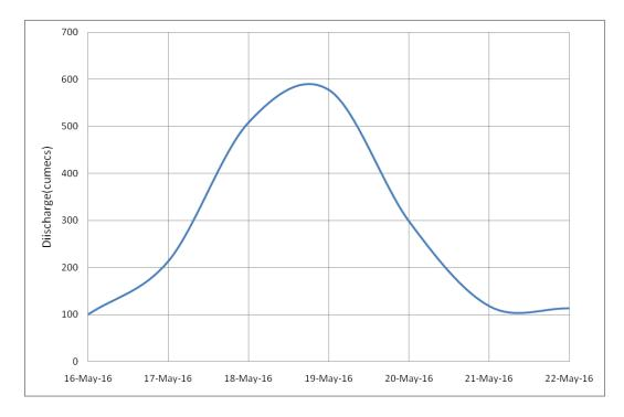
Fig. 5 Computed flood hydrograph of Adyar River in M<sup>3</sup>/Sec (computed as on 19<sup>th</sup> May 2016)
