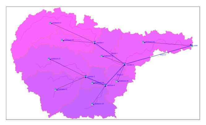
Fig. 3 Basin Model Setup of the Adyar River Catchment
